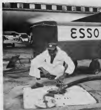
FROM A hydrant, G. T. Walle, Esso aircraft refueler, prepares to gas up a giant airliner. FOR DI un hydrant, G. T. Walle, Esso aircraft refueler, ta prepara pa entrega combustible na un avion.
